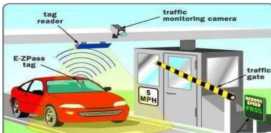
Fig.1 Automatic toll collection system
